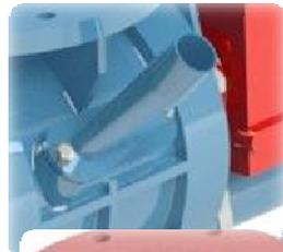
5. Inlet for granulates, grain size >500 µm, cubic up to 10 mm, made of carbon steel
