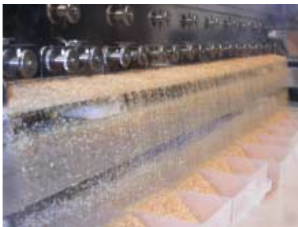
Powdering machine, width 1000 mm.
